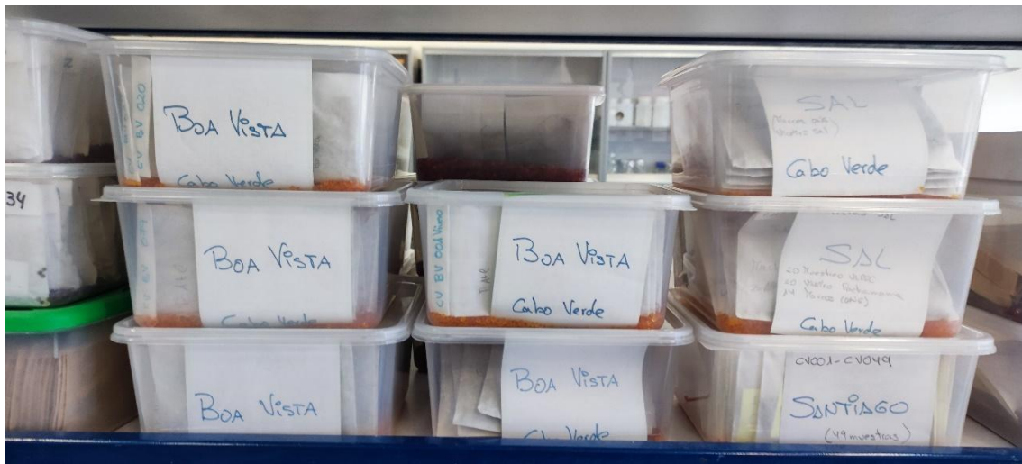
Photo 12. Storage of samples in boxes. It is important to renew the silica gel every six months or as soon as it is observed that the gel has turned.
